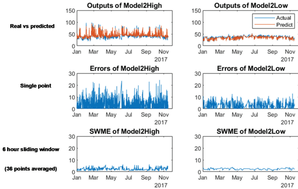
Figure 6. The performance of the model in the training data set time duration including single point and 6 hours sliding window results for both submodels of high and low shaft speeds.
