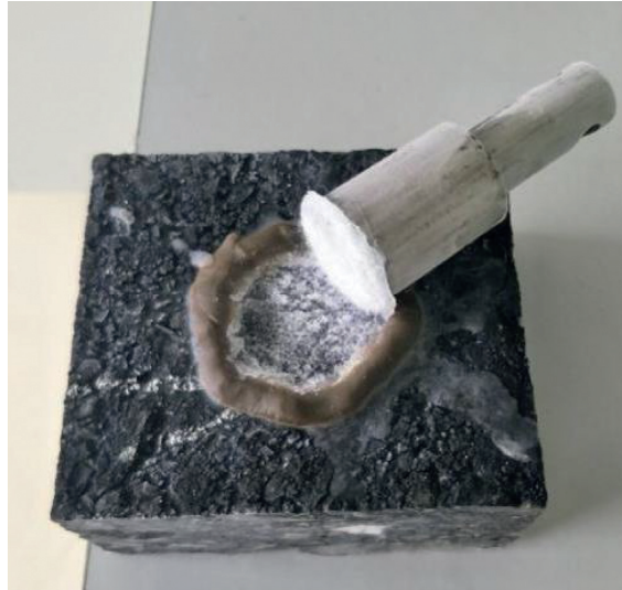
FIGURE 7: Pull-out test to determine tensile force at failure.
